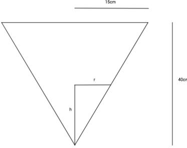
$V_{cono}(r, h) = \frac{1}{3} \pi r^2 h$ $\frac{15}{r} = \frac{40}{h} \Rightarrow r = \frac{3h}{8}$ $V_{cono}(h) = \frac{1}{3} \pi \left(\frac{3h}{8}\right)^2 h = \frac{3\pi}{64} h^3$ |
